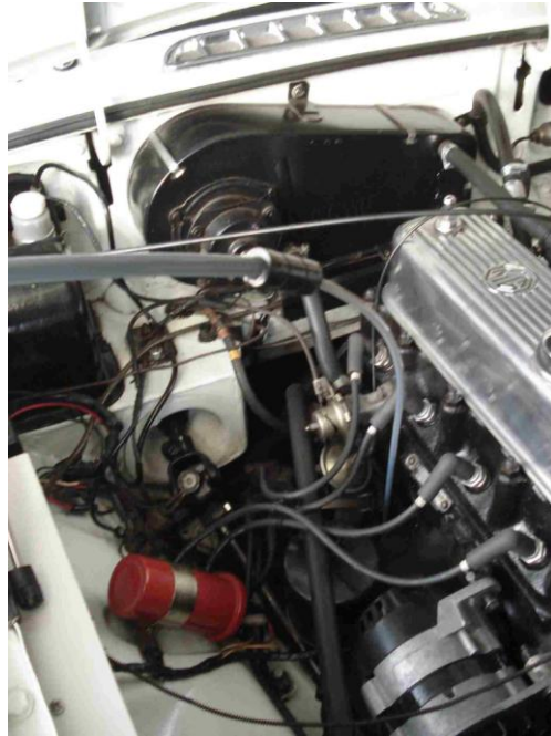
Suction tube going into dipstick tube
