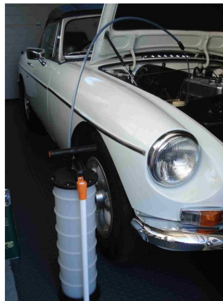
Extractor with suction tube in place
