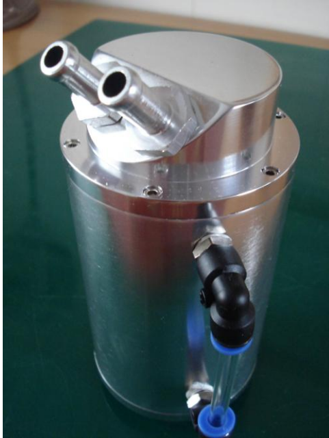
Catch Tank before installation
