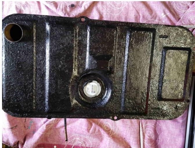
Fig 1. Top of petrol tank showing sender unit (white).
