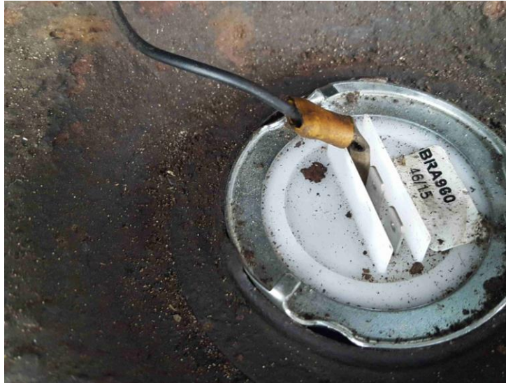
Fig 2. Top of sender unit showing original single connection wire.
