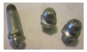
Zerk's nipple overcame this with its tapered head that allowed the gun to attach and lock on even if the approach was less than square. The pressure of the oil or grease then depressed a spring-loaded ball valve to allow lubrication to take place. Once the gun was removed the valve shut to keep lubricant in and dirt out.
