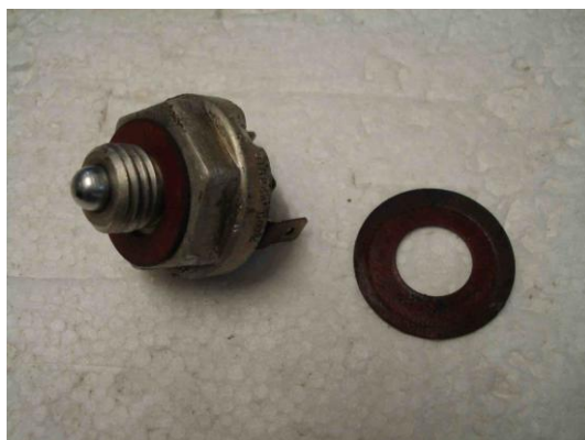
Fig 4. Overdrive inhibitor switch showing one fibre washer removed.
