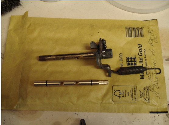
Fig 3. Old throttle shaft and new one with O rings
