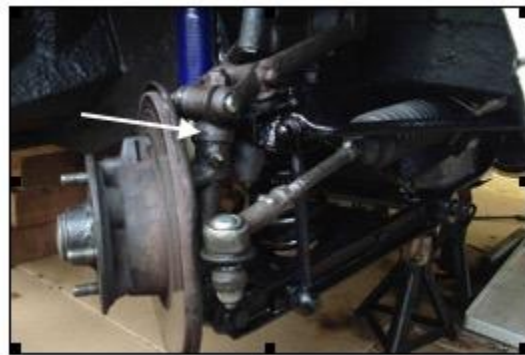
Fig 1. New king pin assemblies. Roller bearing assembly arrowed
