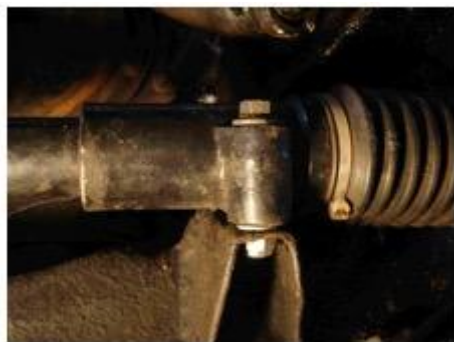
Fig 5. New washers on steering column alignment
