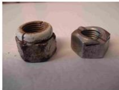
Fig 4. Old (on left) and new (on right) locking nuts
