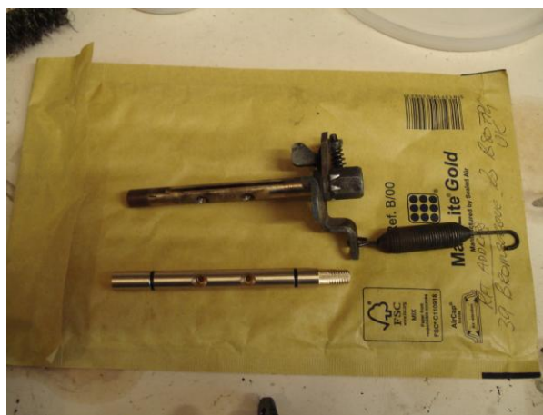
Fig 3. Old throttle shaft and new one with O rings
