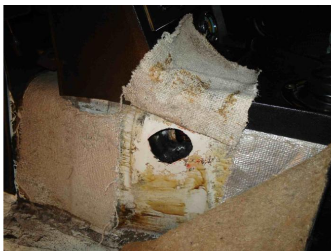
Fig 2. Access hole in transmission tunnel.
