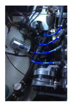
Fig 2. New plug leads and polished coil.
