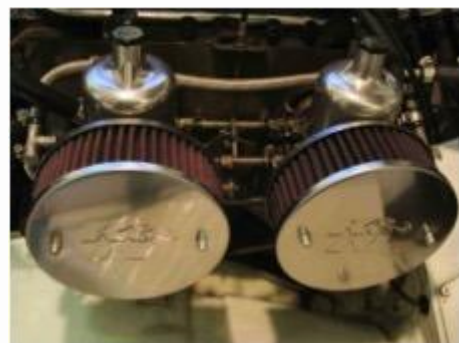
Filters reinstalled (note red colour)
