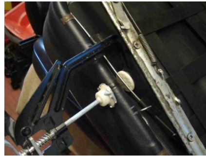
G clamp to assist with new straps
